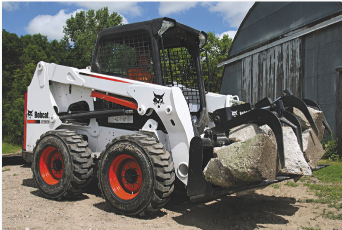
The first skid steer introduced as part of Bobcat's new M-Series loaders, the S630 features the new cab-forward design that both brings the operator closer to the work area and provides the operator with better overall visibility.
